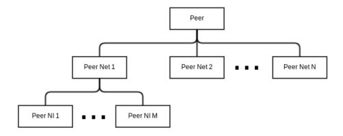
Currently when a route is added the gateway is one of the leaves of the tree, IE a peer NI. To fully integrate routing with MR the gateway should be considered the tip of the tree, IE the peer.
