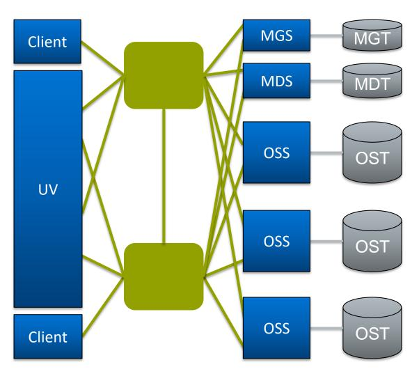
Instead of a router a link connects two fabrics into one LNet network.
